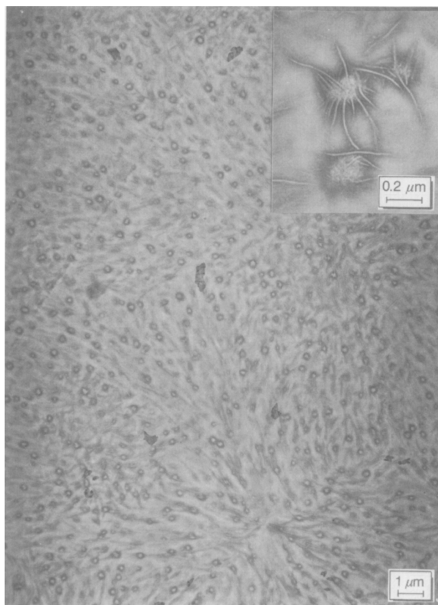
Figure 4 TEM micrographs obtained at position I, showing very small c.s.d.
